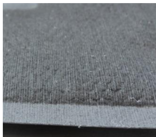
Thinsulate™ Acoustic Insulation RS2400i material
