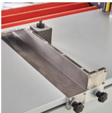
Double magnetic feed guides for sheet feed alignment
