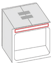
Example of single and double-sided tape application on flat surface
