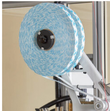
Split spindle for applying two rolls of tape on the same applicator
