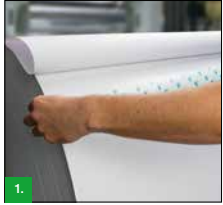
Figure 1 + 2: Apply the tape under the top layer of the paper roll. Remove the upper part of the liner to expose the adhesive.
