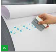
Figure 1 + 2: Apply the tape under the top layer of the paper roll. Remove the upper part of the liner to expose the adhesive.
